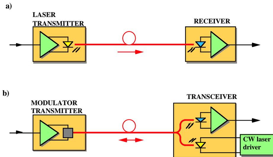
Fig. 3. Two investigated approaches for data transmission: a) direct modulation, b) external reflection modulation
