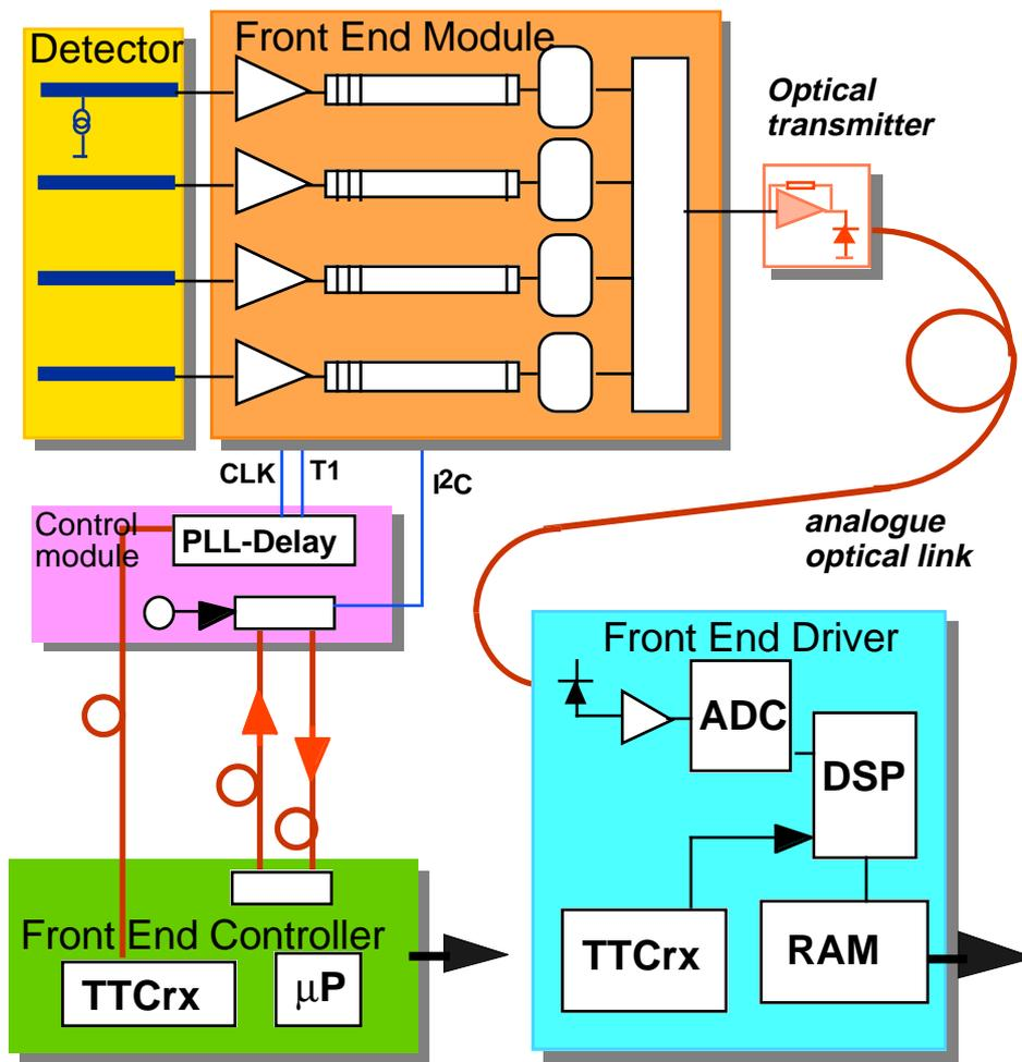
Fig. 1. Simplified schematic of the readout system
