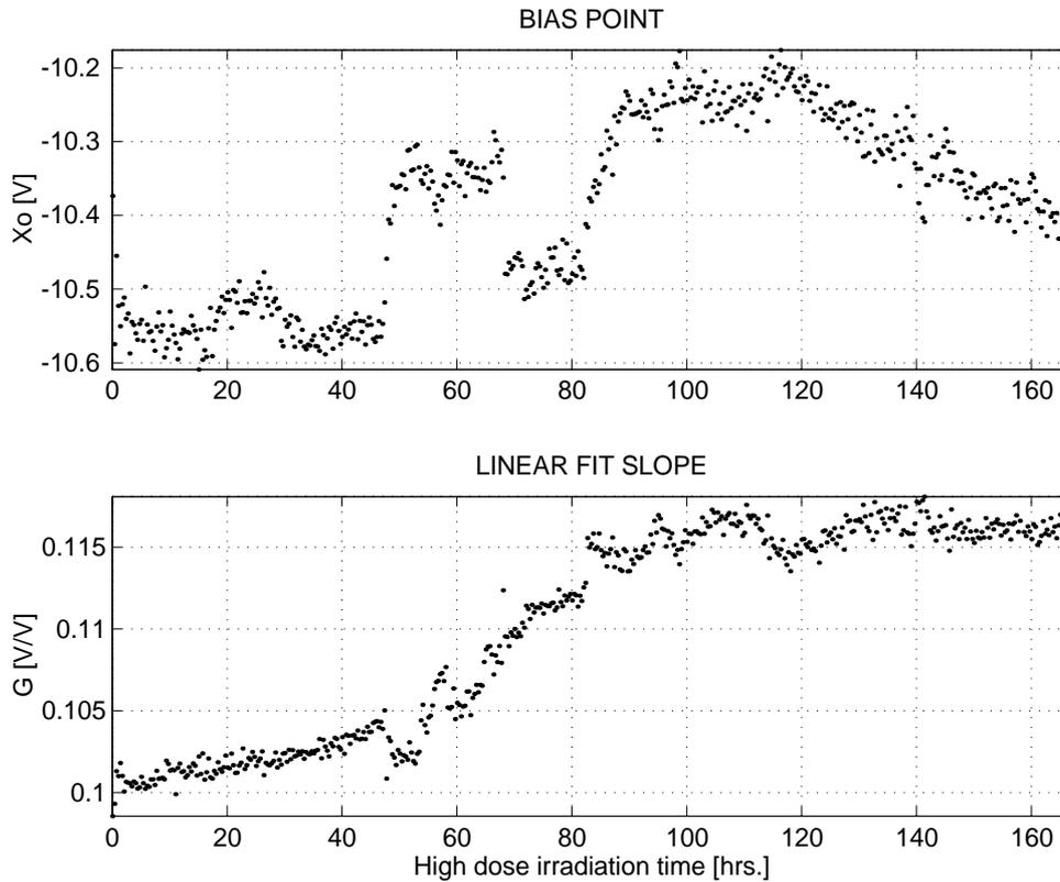
Fig. 9 b) AFPM based link bias point and gain vs time during  $\gamma$  irradiation test
