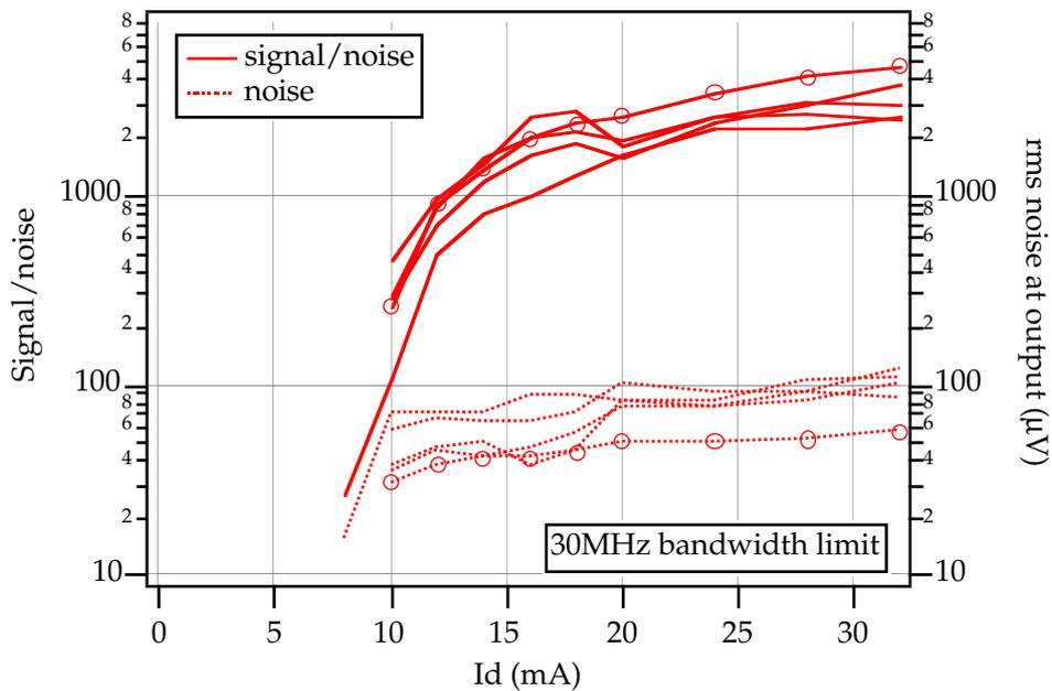
Fig. 5 b) Noise and signal to noise ratio measured in lasers before irradiation.
