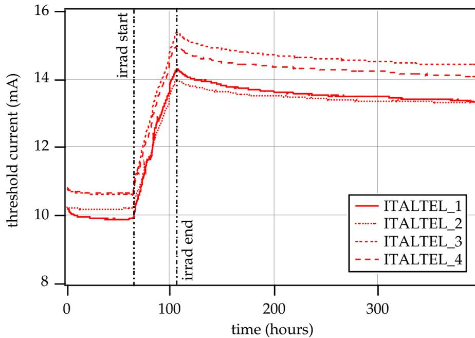
Fig. 7 a) Laser threshold current measured during the irradiation test. The threshold was defined at the point of the transfer characteristic where the output voltage interpolated to 0.05V.
