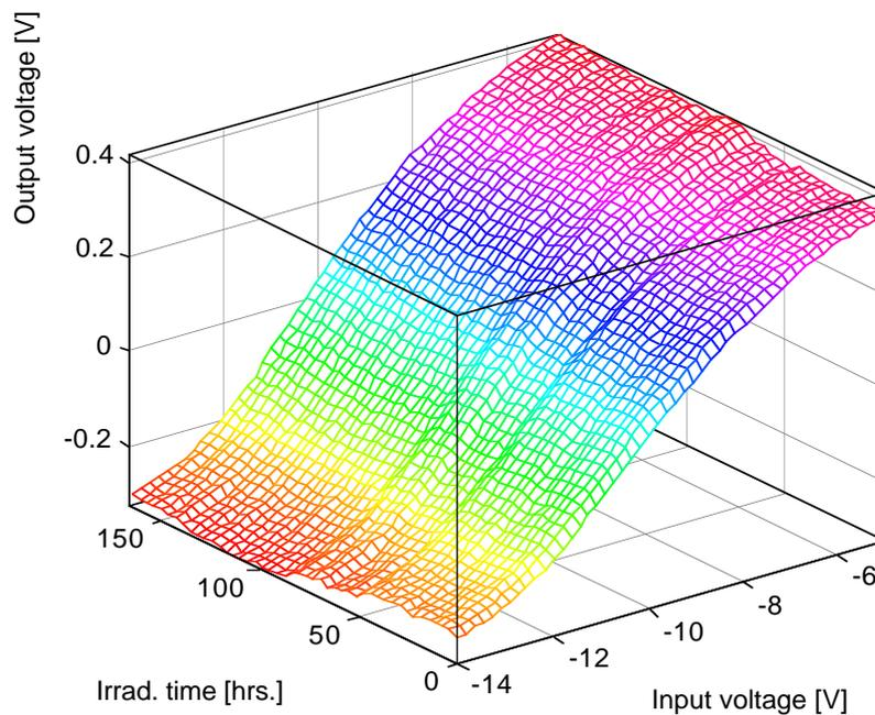
Fig. 9 a) AFPM based link transfer function during  $\gamma$  irradiation test
