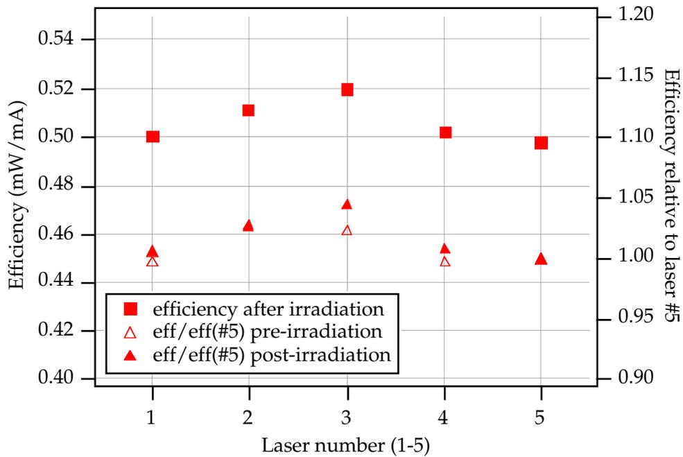
Fig. 8 b) Efficiency (at 22C) from linear fit to transfer characteristics above threshold for lasers of type d) after irradiation. No absolute values for efficiency were available before irradiation therefore the efficiency calculated from the data sheet results normalised to laser #5 was used for comparison with the post irradiation results. Since laser number 5 was not irradiated the results suggest that no radiation damage to the efficiency occurred.
