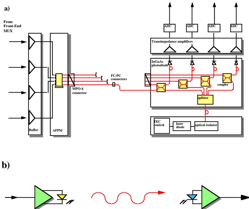
Fig. 4. Experimental set-ups. a) AFPM based link, b) laser transmitter
