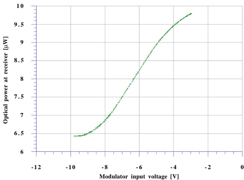
Fig. 6. Reflectance characteristic of AFP Modulator transmitter
