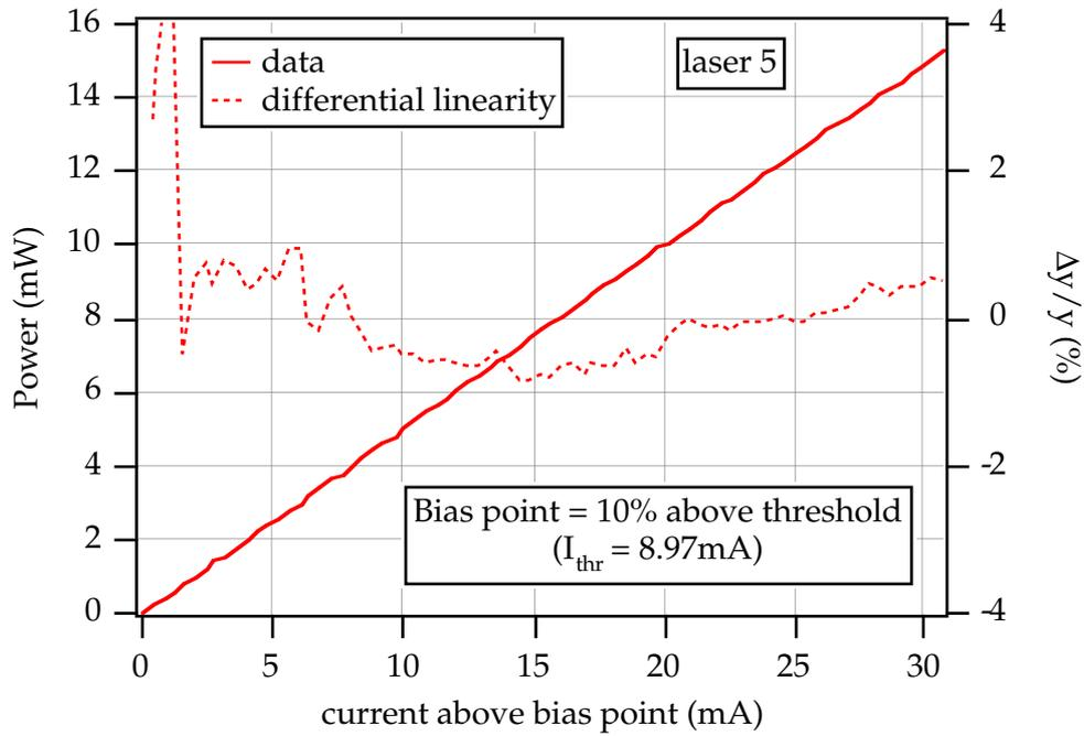
Fig. 5 a) L-I characteristic and differential linearity of laser type (d) above threshold
