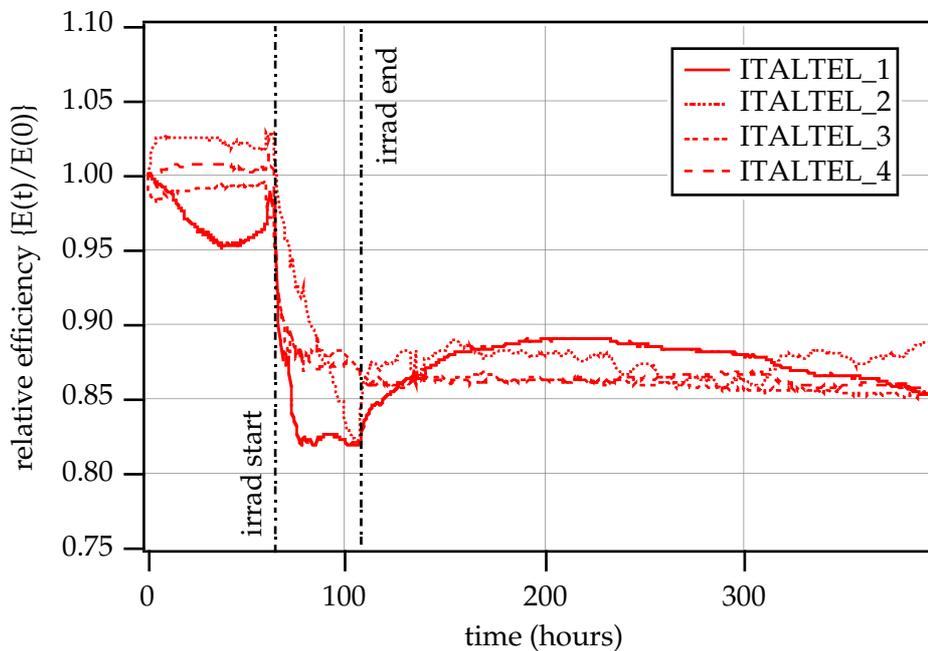
Fig. 7 b) Laser efficiency relative to the start of the test, where efficiency was the gradient of the transfer characteristic at an output voltage interpolated to 0.2V.
