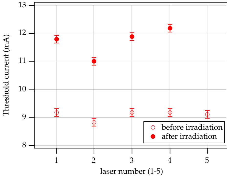
Fig. 8 a) Threshold currents before and after irradiation for lasers of type d). Threshold current in this plot is defined as the peak position in the second derivative of the transfer characteristic. Laser number 5 was not irradiated.
