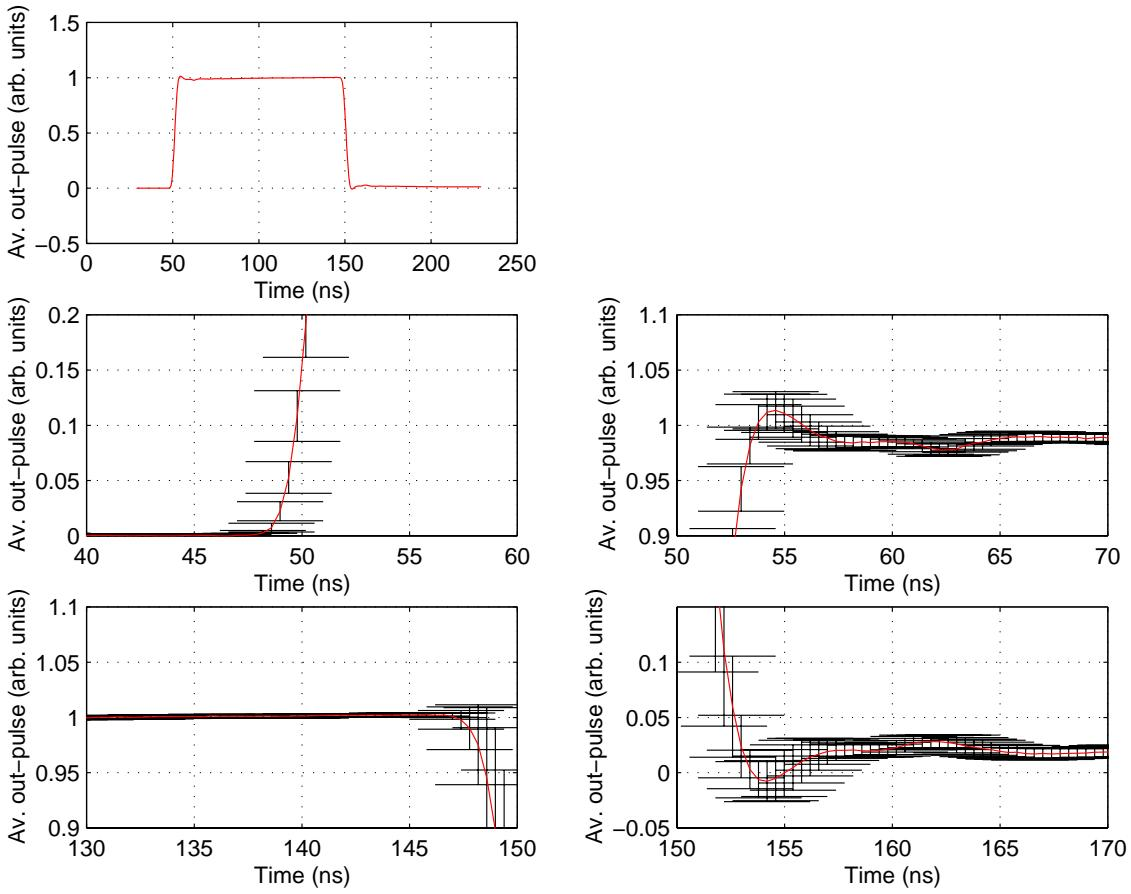
Fig 7: Average and standard deviation of link pulse response over 28 channels. Mean rise-time: 2.87ns.
