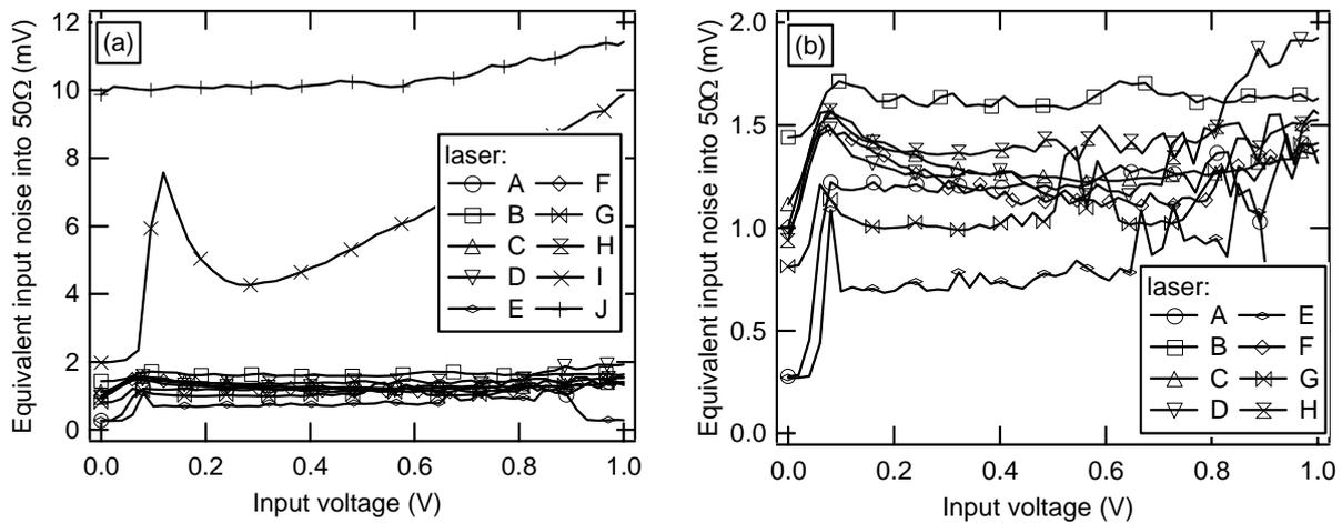
Fig. 4. Equivalent input noise for links with different laser transmitters (a) full set of 10 different lasers. (b) lasers I and J excluded.
