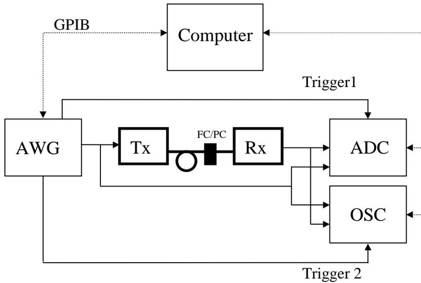
Fig. 2. Experimental setup for link and device performance tests
