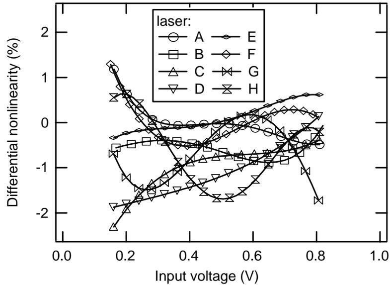
Fig. 5. Differential non-linearity of lasers A-H (laser I, J excluded) as a function of link input voltage. Non-linear regions close to laser threshold and receiver saturation have been excluded.
