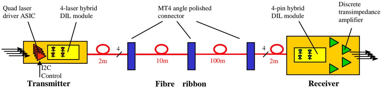
Figure 1. 4-channel optical link prototype
