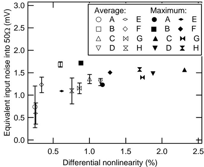
Fig. 6. Average and maximum of equivalent input noise and absolute differential non-linearity for lasers A-H. Error bars give standard deviation of equivalent input noise.
