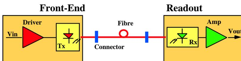
Fig. 1. Generic optical link based on a directly modulated laser transmitter (Tx) and a photodiode receiver (Rx).
