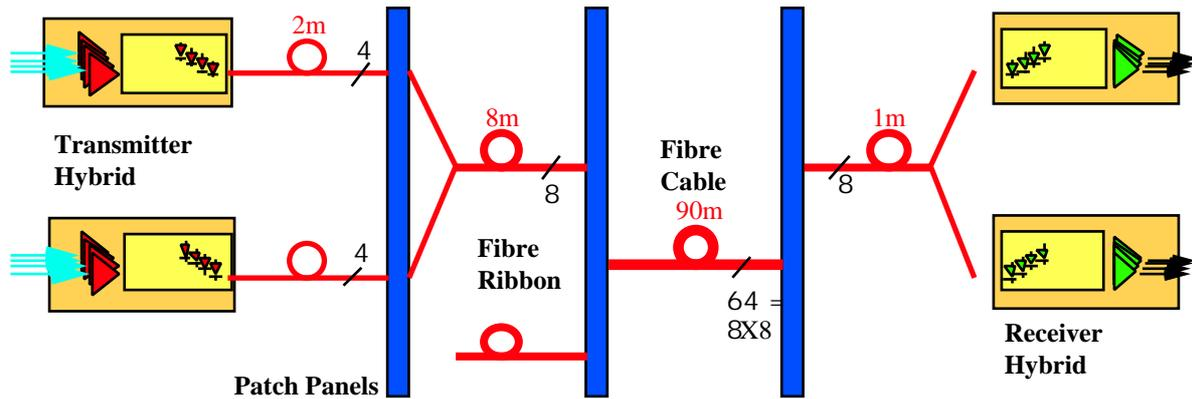
Fig. 3. Analogue optical link layout
