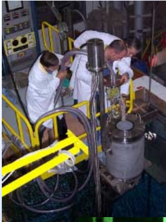
SCK-CEN Co-60 \gamma dose rate 2kGy/hr underwater source
