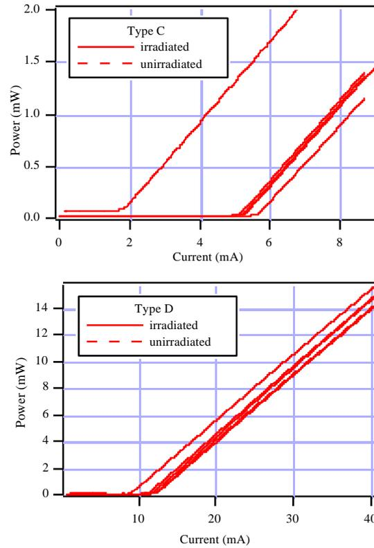
Fig. 7: L-I curves measured in the lab after irradiation.
