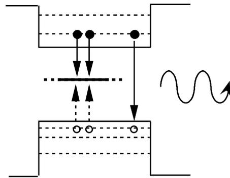
Fig. 10(b): Irradiated QW laser. Recombination competes with lasing transitions.
