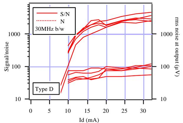
Fig. 3: S/N measurements for type D lasers.
