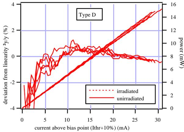
Fig. 9: Linearity measurements for type D lasers.
