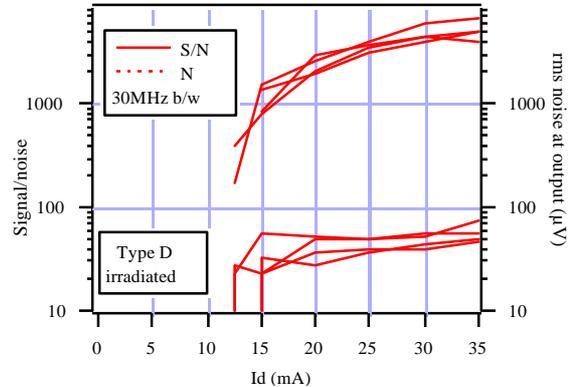
Fig. 8: S/N measurements for type D lasers after irradiation.
