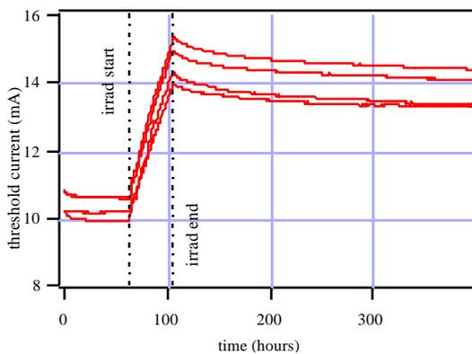
Fig. 5: Change in the laser threshold current for type D lasers.
