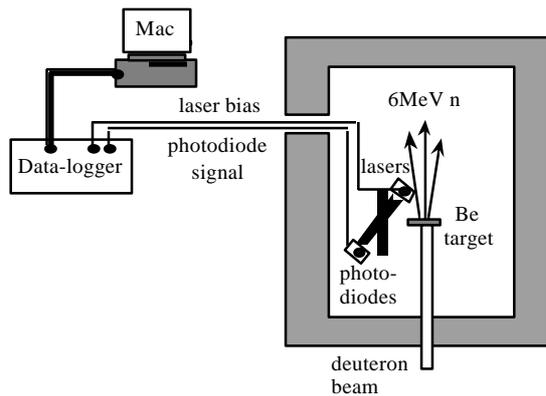
Fig. 1: Schematic experimental arrangement for the neutron irradiation.
