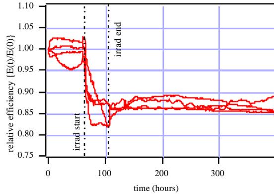
Fig. 6: Change in the laser efficiency for type D lasers.
