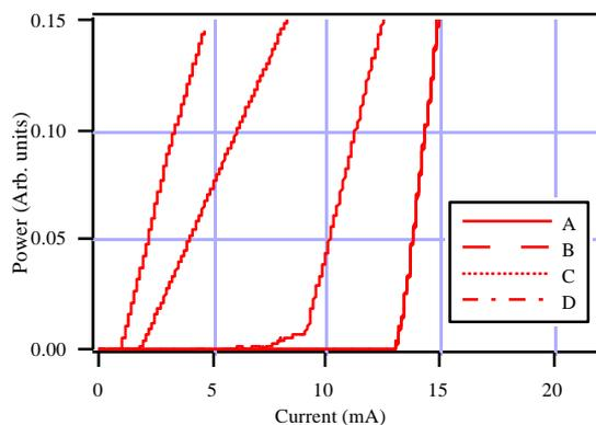
Fig 2: Typical L-I curves for the four laser types.
