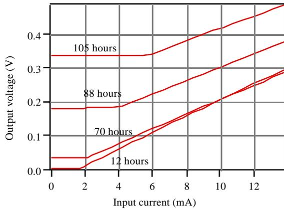
Fig. 4: Sample of results for type C lasers measured during the irradiation test. Irradiation took place between 64 and 107 hours.
